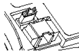
Figure 7: Slave Setting for Vertical iDiskOnChip 40-Pin Connector
