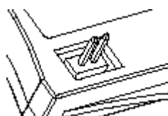
Figure 8: Master Setting for Vertical iDiskOnChip 44-Pin Connector
