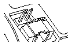
Figure 9: Master Setting for Vertical iDiskOnChip 40-Pin Connector
